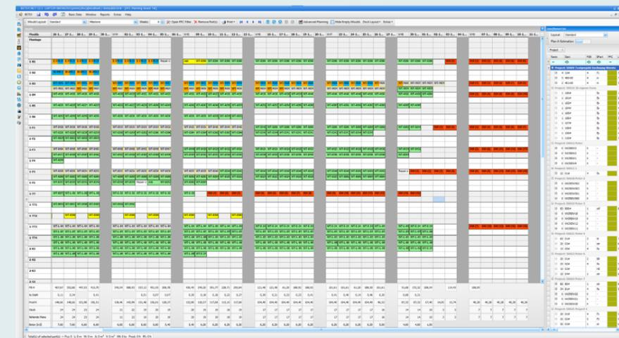
of the labor estimation based on the final element drawings. Assignment of elements to moulds is done via drag and drop. The daily hours required for different production steps, and materials used, are
